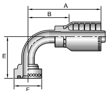
Caterpillar® style fittings conform to the bolt hole patterns of SAE Code 62 and require special flange halves and seals. The Caterpillar® style flange heads are thicker than SAE Code 62 and measure to a .560" thickness in all sizes.
