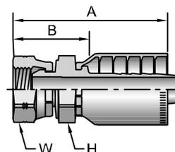
Metric S: Mates with EO "S" Series Fittings. See Accessories Section for O-Rings and Flange Kits.
