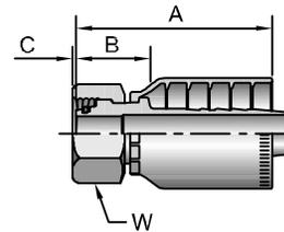
When measuring overall length to the end of the nut, B+C dimensions must be used to calculate cut-off allowance.
