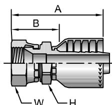
Japanese Fittings - Female Swivel 30° Flare with Metric Threads. All 30° flared fitting sizes are available by combining 1MU71 fittings in sizes up to 1/2 with 1XU71 fittings in sizes 5/8 inch and larger.
