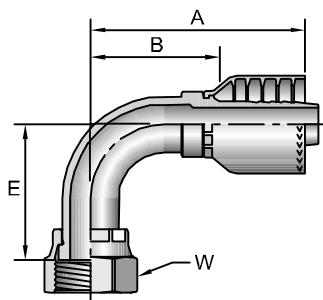
**1J171****Female Seal-Lok® - Swivel - 90° Elbow - Long Drop**
