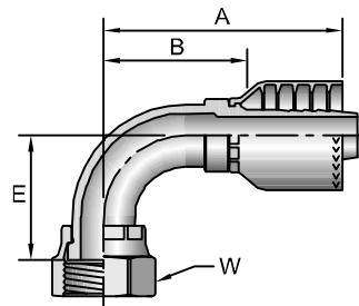
**1J571****Female Seal-Lok® - Swivel - 90° Elbow - Medium Drop**
