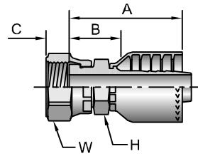
When measuring overall length to end of nut, B+C dimensions must be used to calculate cut-off allowance.
